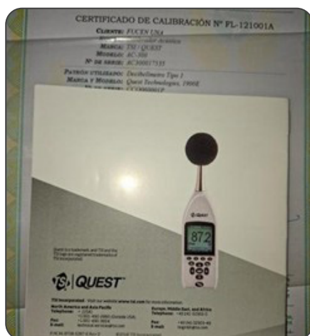
Figure 1: Class 1 sound level meter, used for measurements. Source: own elaboration.
